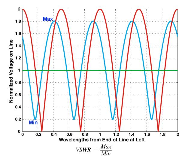
Red Curve: Standing wave on line with open circuit at left end (antenna terminals)
